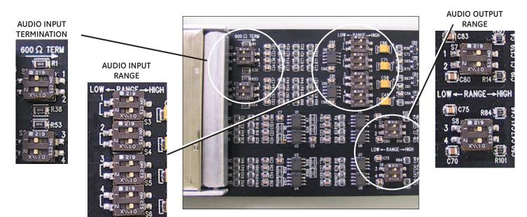
Figure 1. Audio Level Switch Locations
